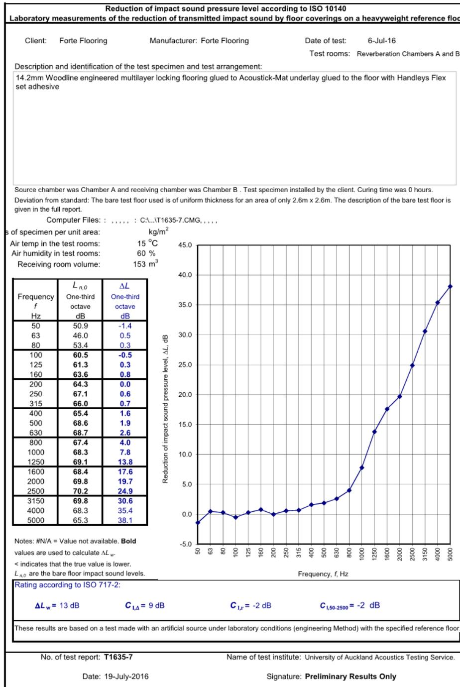
**Table 1: 14.2mm Woodline Engineered multilayer flooring on Acoustick-Mat underlay - Impact Insulation Prediction**
